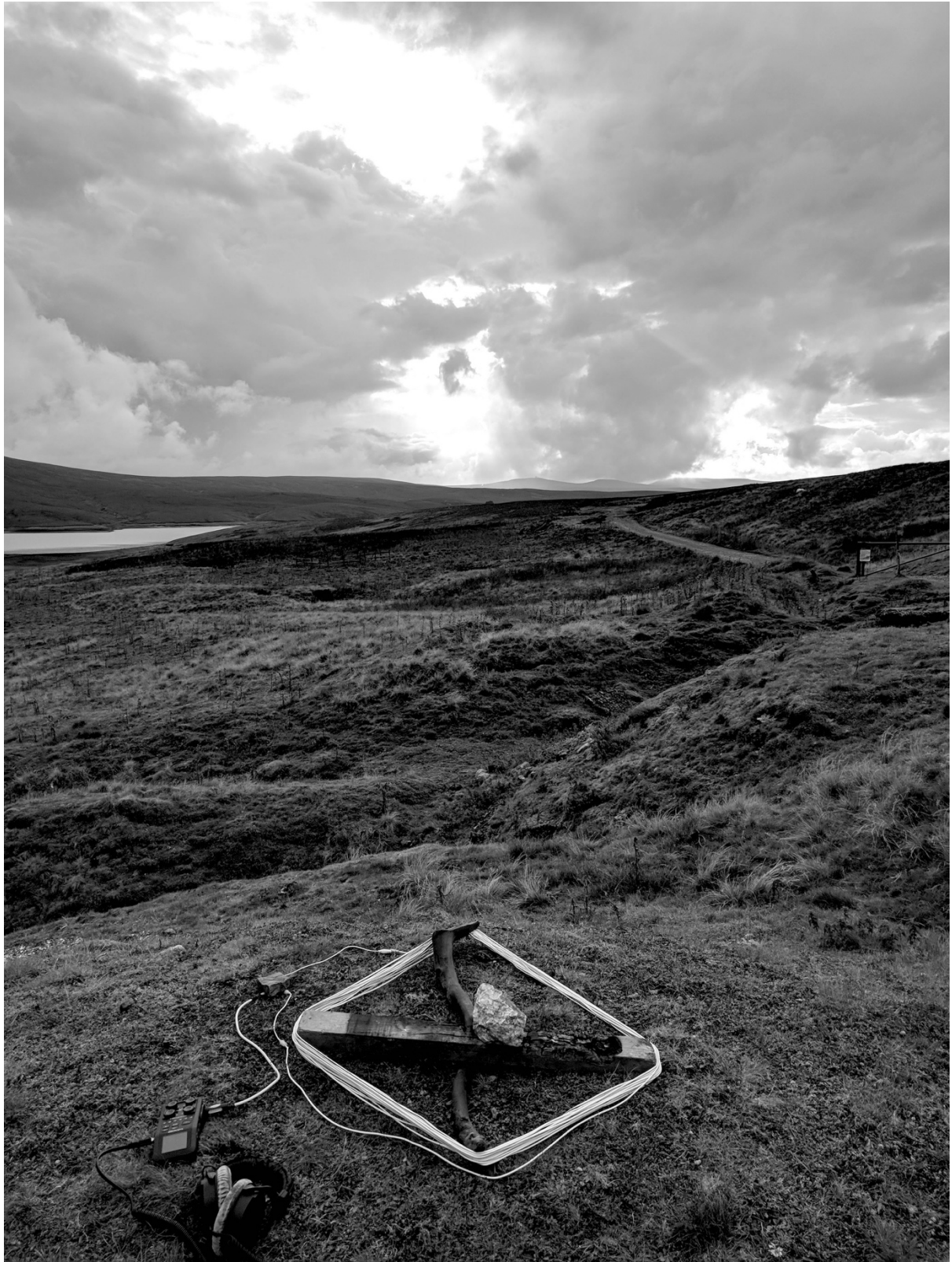
Figure 2 DIY Aerial for Atmospheric Listening
